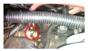
Attach the other end of the ground wire to an empty threaded mount hole that is located right underneath the center of where the stock airbox was prior to removal using a supplied bolt. Check pic below:
