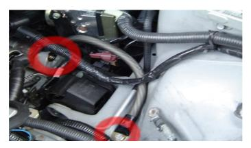
Step four: Using a supplied bolt attach one end of the longest wire in the kit to the empty threaded mount tab located to the driver's side of the oil dip stick on the engine block. Attach the other end of the ground wire to the stock ground point closest to the windshield wiper reservoir.
