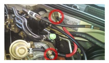
Step two: Take the next to shortest wire supplied in the kit and attach it to the 10mm Bolt attached to a bracket at the top of the timing chain cover. You will notice the bolt is fairly close to two stock grounds. Attach the other end attaches to the empty threaded chassis mount point closest to the passenger's side motor mount using a supplied bolt.
