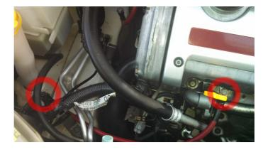
Step five: Take the next to longest wire supplied in the kit and using the supplied nut attach one end to the negative battery post as displayed in the pic below. You will than attach the other end of this wire to the 10mm bolt stock ground point located right behind the driver side headlight.
