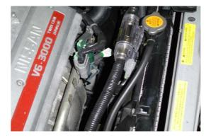
I looped the zip ties around the top plastic radiator mount right around the point the stock power wiring for the fans end. The fuse holder has a mount plate that has four holes that you can use. I use one top on to loop around and under the top plastic radiator mount and I used the two lower holes to loop and attach to the stock fan power wires.
