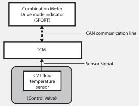
• The CVT fluid temperature sensor detects fluid temperature in the CVT oil pan.
