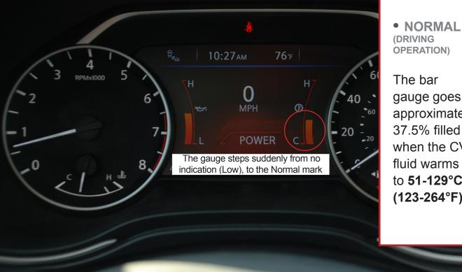
**OPERATION**) The bar gauge goes to approximately 37.5% filled when the CVT fluid warms to 51-129°C (123-264°F).
